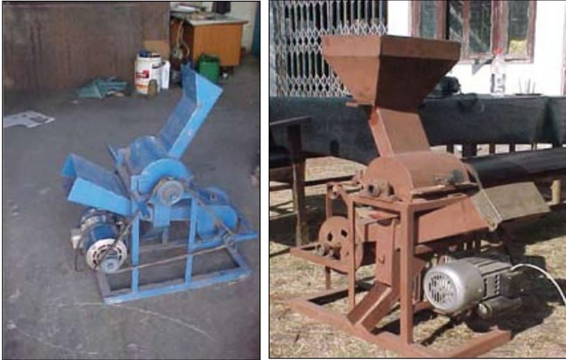
Fig. 15. Millet pearling machine at Kabre (left) and modified pearling machine (right)
