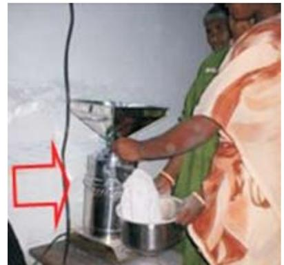
**Fig. 13.** Initially introduced micro-mill for processing finger millet
