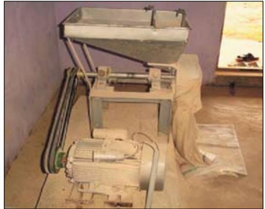
Fig. 14. Power-operated small mill
